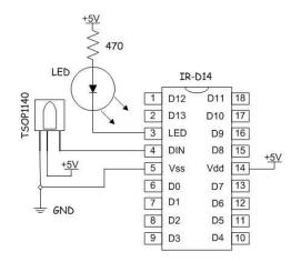
A single 40KHz infrared detector module with the IR-D14 IC completes the entire remote control receiver assembly.
